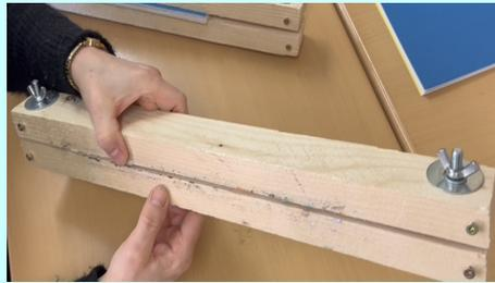
5. Built your own paper presses out of 2 root battens (50 cm long), 2 long wing screws and 4 short screws.
