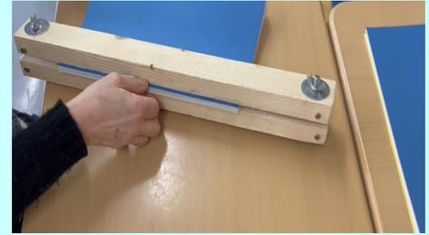
6. Put 4 screws in on one batten to keep a distance from the table.
